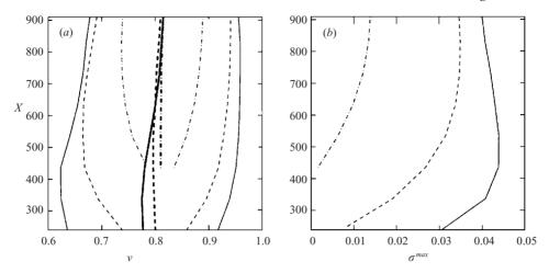
FIGURE 6. Impulse response characteristics of extracted parallel streaks as a function of streamwise distance X for three distinct upstream streak amplitudes at X = 0. A = 0.28: —; A = 0.22: - - -; A = 0.16: · · · · (a) Leading-edge velocity  $v^+$  (thin lines), trailing-edge velocity  $v^-$  (thin lines), centre velocity  $v^{max}$  (thick lines). (b) Maximum temporal growth rate  $\sigma^{max}$ .
