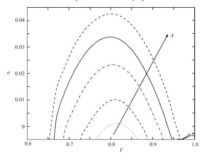
FIGURE 5. Temporal growth rate versus ray velocity x/t = v for different increasing saturated streak amplitudes A = 0.28, 0.31, 0.34, 0.36 and 0.38 at X = 632 and Re = 1047. The solid line corresponds to the base flow at A = 0.36 depicted in figure 1(b) and indicated by an asterisk in figure 1(a). The other curves correspond to scanning the vertical line X = 632 of unstable streaks in figure 1(a) for lower and higher amplitude settings.
