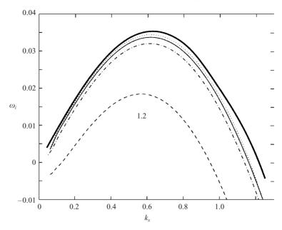
FIGURE 3. Temporal growth rate  $\omega_i$  versus streamwise wavenumber  $k_x$  for the base flow of figure 1(b). The inviscid results of Andersson *et al.* (2001) are represented by the thick solid line: -; Re = 1047: -; Re = 2000:  $\cdots$ ; Re = 500: -; Re = 100: - - -
