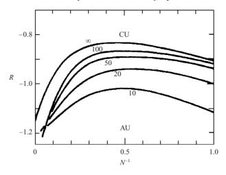
FIGURE 8. Absolute/convective instability boundary in the  $(N^{-1}, R)$ -plane at various wake Reynolds numbers indicated near the curves for the wake profile family (4.2). AU and CU denote the domain of absolute and convective instability, respectively. After Monkewitz (1988).
