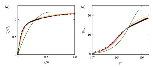
FIGURE 9. (Colour online) Mean streamwise velocity profile  $\bar{u}$  as a function of the wallnormal distance y in bulk (a) and wall units (b). The colour scheme is the same as in figure 6, with the addition of the black symbols used for the Newtonian case, taken from the results by Kim et al. (1987). The viscosity ratio  $\beta$  is fixed equal to 0.95.
