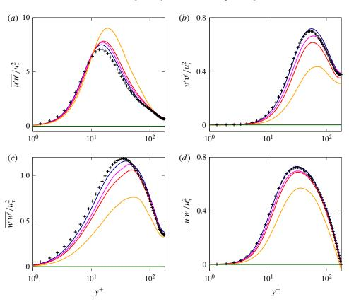
FIGURE 10. (Colour online) Wall-normal profiles of the different components of the Reynolds stress tensor, normalized with  $u_{\tau}^2$ . (a-c) Show the diagonal components u'u', v'v' and w'w', while (d) shoes the cross-term u'v'. The colour scheme is the same as in figure 6.
