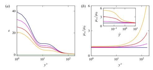
FIGURE 12. (Colour online) Wall-normal profiles of (a) the turbulent dissipation  $\varepsilon =$  $\mu \partial u'_i / \partial x_i \partial u'_i / \partial x_i$  in wall units and of (b) the shear effective viscosity  $\mu_e$ . The colour scheme is the same as in figure 6. The inset figure in (b) shows  $\mu_e$  as a function of the shear rate  $\dot{\gamma}$ .
