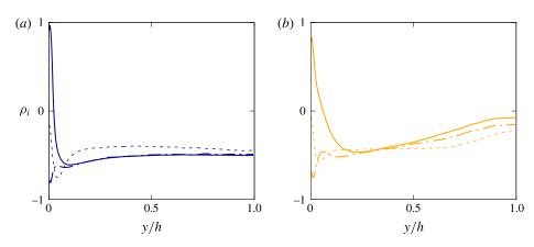
FIGURE 15. (Colour online) Wall-normal profiles of the cross-correlations  $\rho_i$  of the streamwise (dashed line), wall-normal (solid line) and spanwise (dash-dotted line) velocity component  $u_i$  and elastoviscoplastic contribution  $f_i$ , defined in (3.5), for (a) Bi = 0 and (b) Bi = 1.4.
