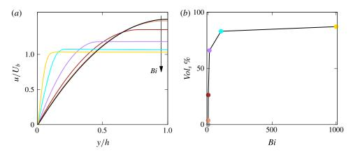
FIGURE 4. (Colour online) (a) Mean streamwise velocity profile  $\bar{u}$  as a function of the wall-normal distance y. (b) Percentage of the unyielded volume  $Vol_s$  as a function of the Bingham number Bi. The Reynolds number is equal to 1, and the colour scheme is the same as in figure 3. Note that, the lines in the graphs are simple connections between the available data points.
