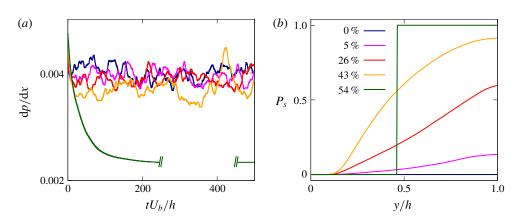
FIGURE 6. (Colour online) (a) Time history of the streamwise pressure drop dp/dx for different Bingham numbers Bi. (b) Probability of the fluid being unyielded  $P_s$  as a function of the wall-normal distance y. The percentages reported in the legend show the mean unyielded volume Vol<sub>s</sub>. The blue, magenta, red, orange and green colours are used for Bi = 0, 0.28, 0.7, 1.4 and 2.8, respectively. The viscosity ratio  $\beta$  is fixed equal to 0.95.
