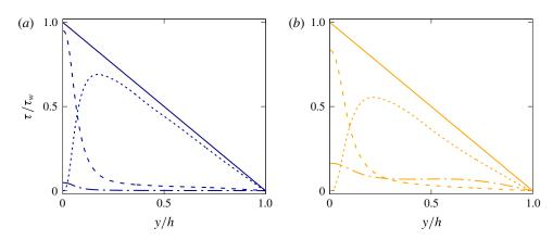
FIGURE 14. (Colour online) Normalized shear stress balance across the channel, for (a) Bi = 0 and (b) Bi = 1.4. The dashed, dotted and dash-dotted lines are used for the viscous, Reynolds and elastoviscoplastic shear stress, respectively, while the solid line is the total shear stress, which varies linearly across the channel height.
