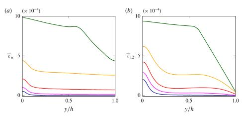
FIGURE 13. (Colour online) (a) Trace and (b) shear component of the mean elastoviscoplastic stress tensor  $\overline{\tau}_{ii}$  as a function of the wall-normal distance y. The colour scheme is the same as in figure 6.
