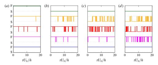
FIGURE 8. (Colour online) Intermittency of the yield/unyield process (F/S) as a function of time. The four panels correspond to probes located at x = 3h, z = 1.5h and different wall-normal distances: (a)  $y \approx 0.25h$ , (b) 0.49h, (c) 0.74 and (d) 0.98h. The lines in every panel are the results with different Bingham number, with the colour scheme being the same as in figure 6.
