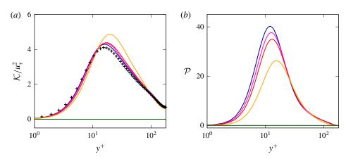
FIGURE 11. (Colour online) Wall-normal profiles of (a) the turbulent kinetic energy  $\mathcal{K} =$  $(u^2 + v^2 + w^2)/2$  and of (b) the turbulent production  $\mathcal{P} = -\overline{u'v'}\,d\overline{u}/dy$ , both normalized with the friction velocity  $u_{\tau}$ . The colour scheme is the same as in figure 6, with the blue, magenta, red, orange and green colours used for the turbulent cases with Bi = 0, 0.28, 0.7, 1.4 and 2.8, respectively.
