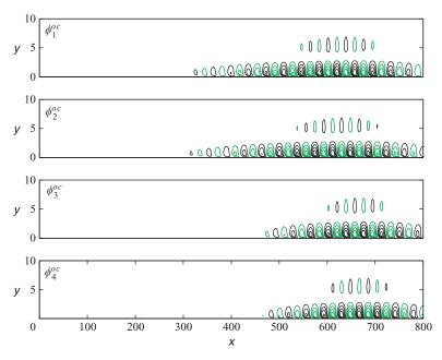
FIGURE 8. The streamwise velocity component of the first four balanced modes  $\phi_i^{oc}$ .
