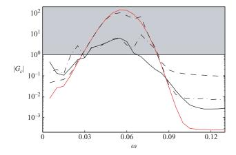
FIGURE 16. Comparison of the frequency response from disturbances to objective function  $(\mathcal{B}_1 \to \mathcal{C}_1)$  of open-loop (red) and three closed-loop systems. The cheap, intermediate and expensive controllers are represented by the solid black, dashed-dotted and dashed lines respectively. The infinity norm of the open loop is  $\|G\|_{\infty}$  is 140.7, whereas for the closed-loop systems  $\|G_c\|_{\infty}$  it is 6.4 (cheap), 9.4 (intermediate) and 101.9 (expensive).
