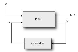
FIGURE 13. The closed-loop system. The plant represents the input-output system given by (2.12) subject to external disturbances w. The controller of the order 50 forces the Navier-Stokes equations with the input signal u based on the noisy measurements v, so that the effect of w on the output signal z is minimized.
