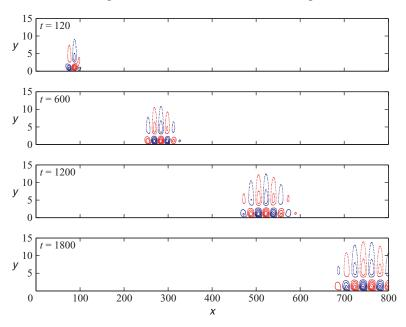
FIGURE 3. Instantaneous snapshots of the streamwise disturbance component at t = 120, 600, 1200 and 1800 triggered by an impulse in  $\mathcal{B}_1$ .
