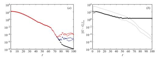
FIGURE 10. (a) The Hankel singular values (black symbols) are compared to the diagonal entries of the controllability (red) and observability (blue) Gramians associated with the balanced reduced-order system. (b) The  $\mathcal{H}_{\infty}$  model reduction error. The upper and lower theoretical bounds are depicted with grey lines, and the actual model reduction error is shown with black symbols.
