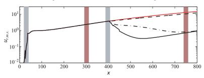
FIGURE 15. The r.m.s. values of the uncontrolled system (red line), cheap controller (solid black), intermediate controller (dashed-dotted line) and expensive controller (dashed line). The grey bar represent the size (defined as 99 % of the spatial support) and the location of the two inputs, whereas the red bars correspond to the two outputs.
