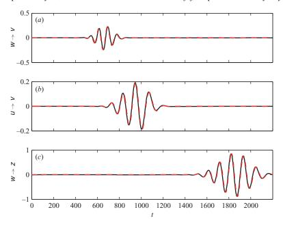
FIGURE 11. The impulse response from  $\mathcal{B}_1 \to \mathcal{C}_2$  (a),  $\mathcal{B}_2 \to \mathcal{C}_1$  (b) and  $\mathcal{B}_1 \to \mathcal{C}_1$  (c). The black solid line represents direct numerical simulations with  $10^5$  degrees of freedom and the red dashed line the balanced reduced-model with 50 degrees of freedom.
