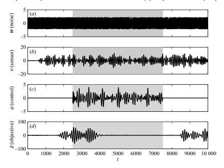
FIGURE 14. Input and output signals of the closed-loop system. The (a) random forcing w, (b) measurements signal v, (c) control signal u and (d) objective function z are shown. The cheap controller is active between  $t \in [2500, 7500]$ , represented by the grey area.
