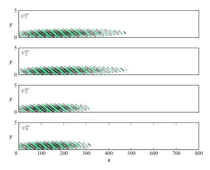
Figure 9. The streamwise velocity component of the adjoint balanced modes  $\psi_i^{oc}$ .
