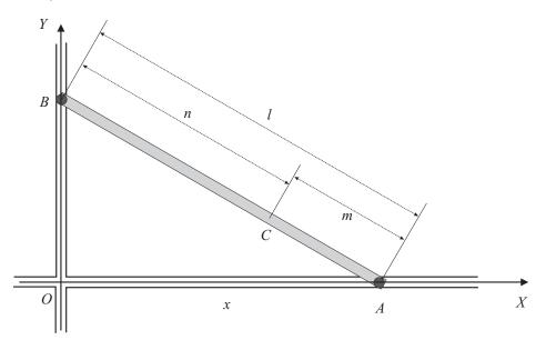
**Hints**: You could use the formula connecting the velocities of different points in a rigid body directly. It is, however, simpler to use the fact that there is pure rotation about the instantaneous center of zero velocity. You then also need the cosine theorem to get the length to C.
