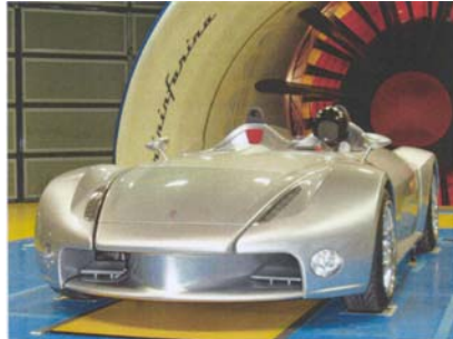
Buffeting around the driver's head using a "Comfort Helmet"
