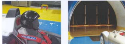
Buffeting around the driver's head using a "Comfort Helmet"
